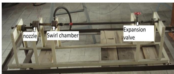
Fig 1. Experimental set up of vortex tube
